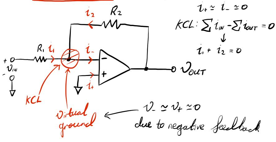
The non-inverting input is connected to ground and a pair of resistors,  $R_1$  and  $R_2$  (the feedback resistor) is used to define the gain. To simplify the analysis we make the following assumptions:
