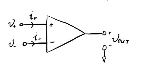
• The op-amp is basically a "three terminal" signal amplifier with two inputs and an output. It is a differential amplifier with very high gain, A, (typically  $10^4$  to  $10^5$ ). The two inputs are known as the non-inverting  $(v^+)$  and inverting  $(v^-)$  inputs respectively. In the ideal op-amp we assume that the gain A is infinite.
