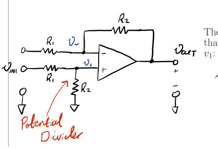
The analysis is simplified by the presence of negative feedback so that  $v^+ \approx v^-$ . The voltage at  $v^+$  is given by potential division of  $v_1$ :
