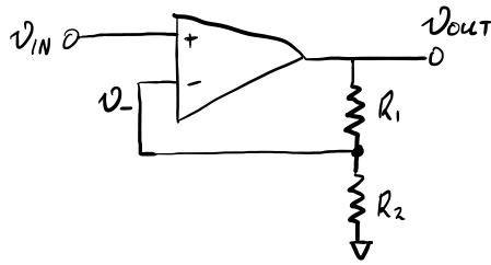
$$U_{-} = U_{\text{out}} \frac{R_2}{R_1 + R_2}$$
