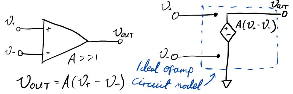
The analysis of op-amp circuits with NEGATIVE FEEDBACK is made significantly simpler by the following approximation which states that the positive and negative input terminal voltages of the op-amp are approximately equal in value.
