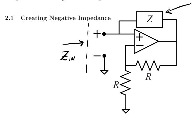
We are interested in determining the input impedance under sinusoidal steady state conditions seen from the input terminals in the circuit above. To do this, we will use complex coefficients to represent the voltages and currents, and complex impedances to represent the passive elements. Then, we apply a test voltage source at the input terminals. The general impedance, Z, might be a capacitor, an inductor or a resistor.
