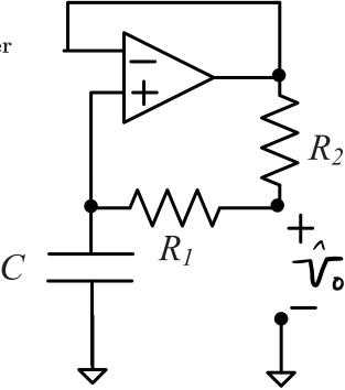
The circuit above can be used to increase the apparent value of the capacitor, C, as measured at the output terminals labeled + and -. Again, we will analyse the circuit using impedance analysis and calculate the output impedance with the application of a test voltage source.
