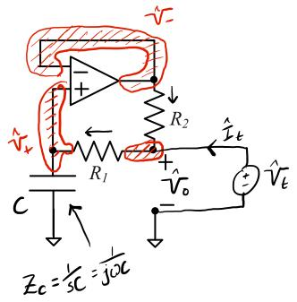
$$Z_{o} = \frac{R_{2}}{J \Omega C(R_{1}+R_{2})} + \frac{R_{1}R_{2}}{R_{1}+R_{2}}$$
