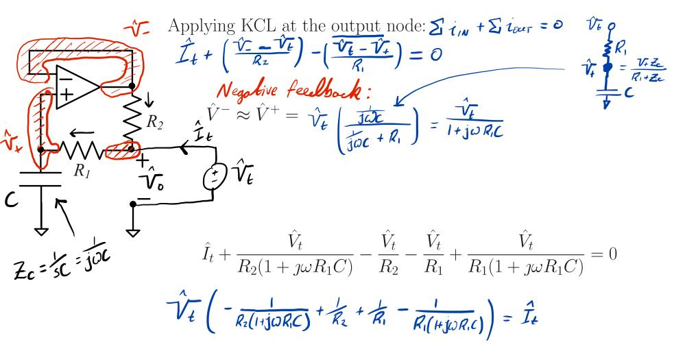
$$\frac{1}{\hat{Z}_{O}} = \frac{\hat{I}_{t}}{\hat{V}_{t}} = \frac{-R_{1} + R_{1}(X + \jmath\omega R_{1}C) + R_{2}(X + \jmath\omega R_{1}C) - R_{2}}{R_{1}R_{2}(1 + \jmath\omega R_{1}C)}$$
