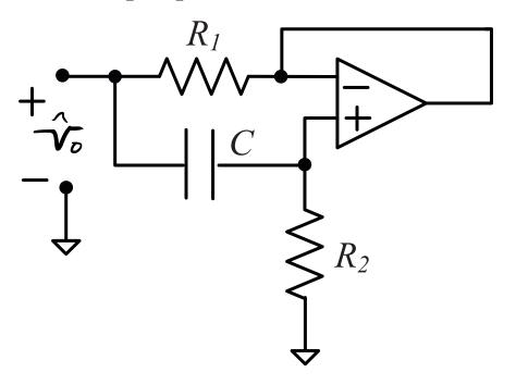
Again, we analyse the circuit using complex analysis and calculate the apparent input impedance,  $\hat{Z}_{in}$ .
