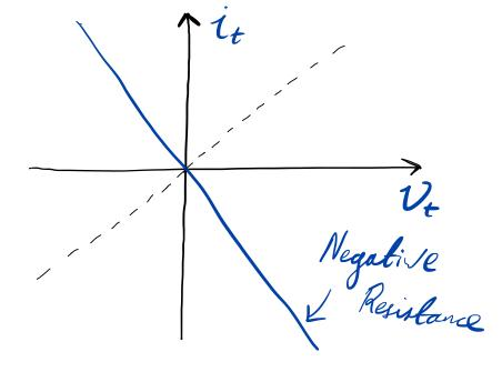
While not common, negative resistors do occur. Fluorescent lamps have negative differential resistance which is electrically balanced with a ballast which adds positive impedance to the circuit. The ballast counteracts the negative resistance of the tube, thus limiting the current in the lamp.
